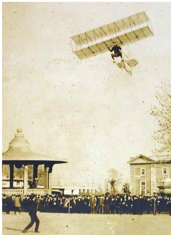
FRANK AVERY. IN AN AEROPLANE. TWENTY-FIVE FEET ABOVE THE PLAZA OF ST. LOUIS. PHOTOGRAPHED YESTERDAY AFTERNOON JUST BEFORE THE AEROPLANE FELL TO THE GROUND, OWING TO THE BREAKING OF A PULL ROPE WHICH WAS TO HAVE STEADIED THE MACHINE UNTIL MR. AVERY HAD ATTAINED THE HEIGHT HE WISHED TO GO BEFORE SOARING.
